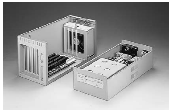
The IPC-644 is an ideal chassis for embedded systems. It can be equipped with 4-ISA, 4 PCI or 1ISA/2PCI/1NLX backplanes to hold up to 4 half-sized cards. An 80 W power supply is included.
