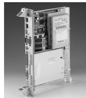
The MIC-3365 with on-board HDD and FDD
