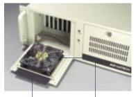
Easily replaceable cooling fan and filter
