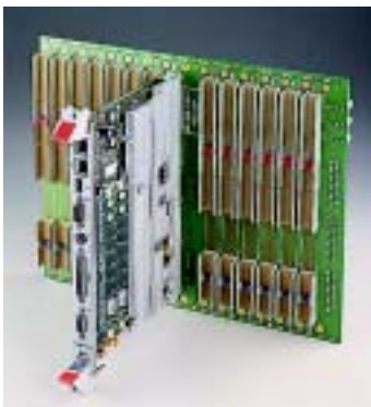
Dual PCI-to-PCI bridge drives up to 14 bus master PCI slots (MIC-3365D)
