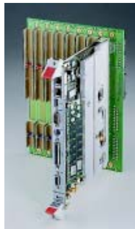
Single PCI-to-PCI bridge drives up to 7 bus master PCI slots
