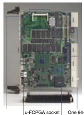
u-FCPGA socket One 64-bit/66 MHz One CompactFlash PMC connector socket Memory on board One 2.5" IDE socket
