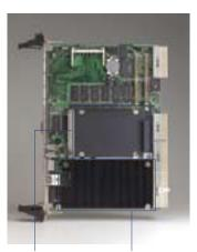
One 2.5" HDD bay One passive CPU heatsink
